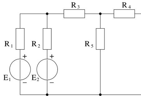
$$\begin{aligned} R_1 &= 1\text{K}\Omega \\ R_2 &= 3\text{K}\Omega \\ R_3 &= 5\text{K}\Omega \\ R_4 &= 2\text{K}\Omega \\ R_5 &= 3\text{K}\Omega \\ E_1 &= 5\text{V} \\ E_2 &= 15\text{V} \end{aligned}$$
