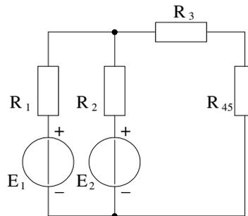
$$R_{45} = \frac{R_4 R_5}{R_4 + R_5} = \frac{2 \times 3}{2 + 3} = 1,2\text{K}\Omega$$
